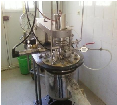
Fig (2) – The device used for determining kinetics of reaction
